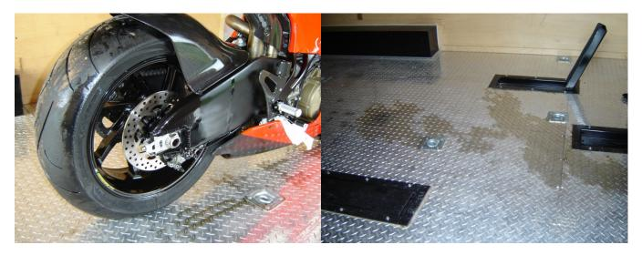
Motorcycle directly after accident in the motorcycle trailer (left). After the motorcycle was removed, synthetic oil was left on the diamond plate floor (right).
