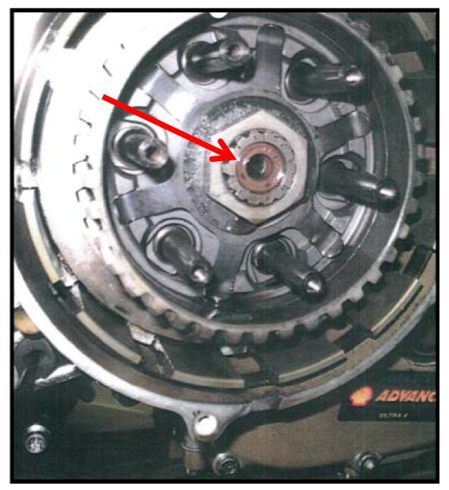
This photo of the clutch cavity shows the failed seal called out with a red arrow and the leaking synthetic oil. Note that the failed seal looks very much like a conventional plumbing washer. The housing, clutch push rod, friction and steel clutch discs, pressure pad and other components have been removed.
