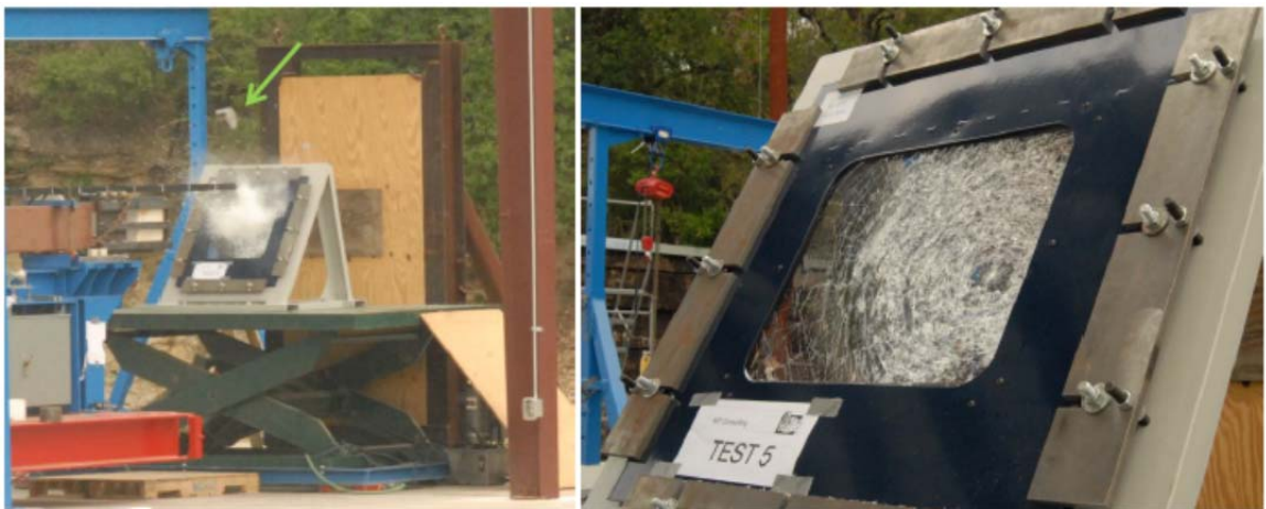
Images from lathe window test. Top – Pneumatic gun for launching workpieces. Lower Left – tested window with rebounding workpiece. Lower Right – Condition of window post Test 5.
