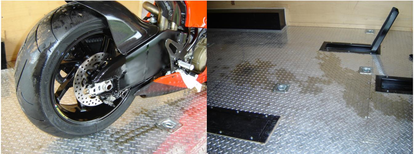
Motorcycle directly after accident in the motorcycle trailer (left). After the motorcycle was removed, synthetic oil was left on the diamond plate floor (right).
